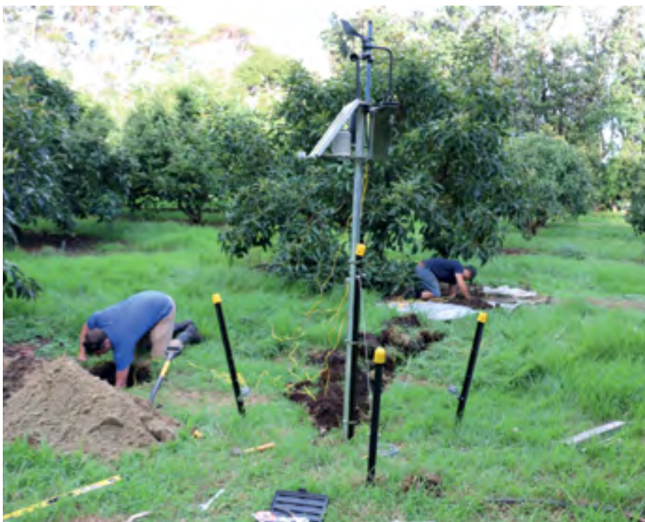
A weather station and soil moisture monitoring being installed in an Avocado orchard.
