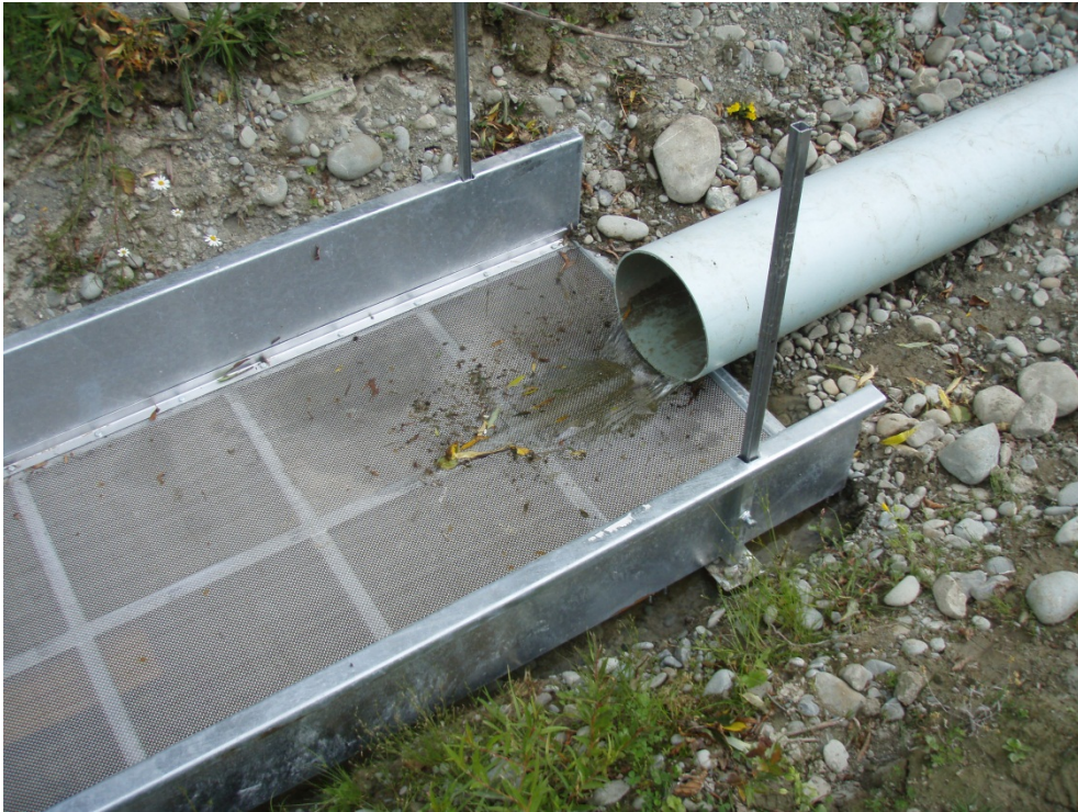
Figure 2-9: The bypass trap. This trap was installed directly downstream of the pipe outlet into the bypass channel.
