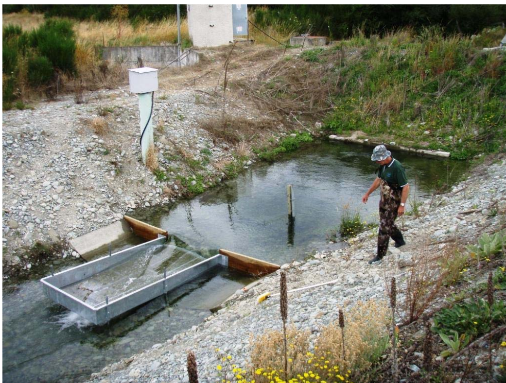
Figure 2-8: The scheme trap. Water passing through the Andar screen (out of picture to right) flowed under the gravel into the scheme channel and then through the trap.
