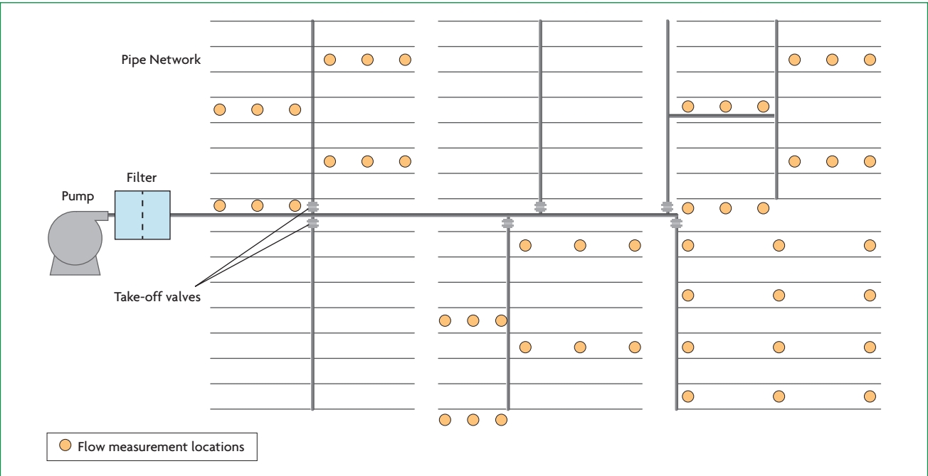
Figure 3.3. Recommended locations for emitter or sprinkler flow measurements for micro-irrigation calibration.
