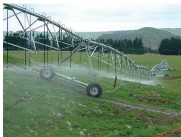
Figure 4. Very steep areas exacerbate surface run-off and apply high loads to machine components including gearboxes
