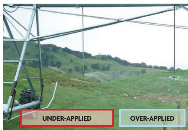
Figure 3. Half-circle sprays direct water away from pivot tower
