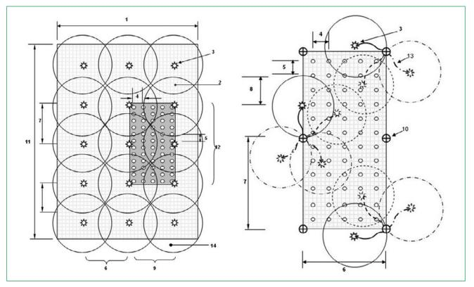
Figure 3.1. Location of sampling grid withing a solid-set irrigation area and withing a long-lateral system
