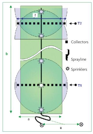
Figure 2.1. Sprayline calibration layout
