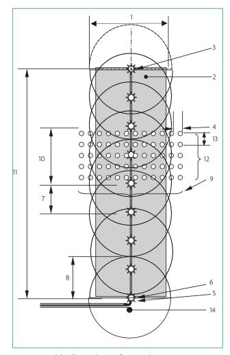
Figure 3.1. Field collector layout for sprayline systems
