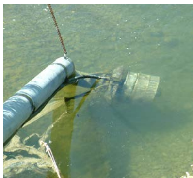
Figure 12. Surface intake using rotating screen to clear debris.
