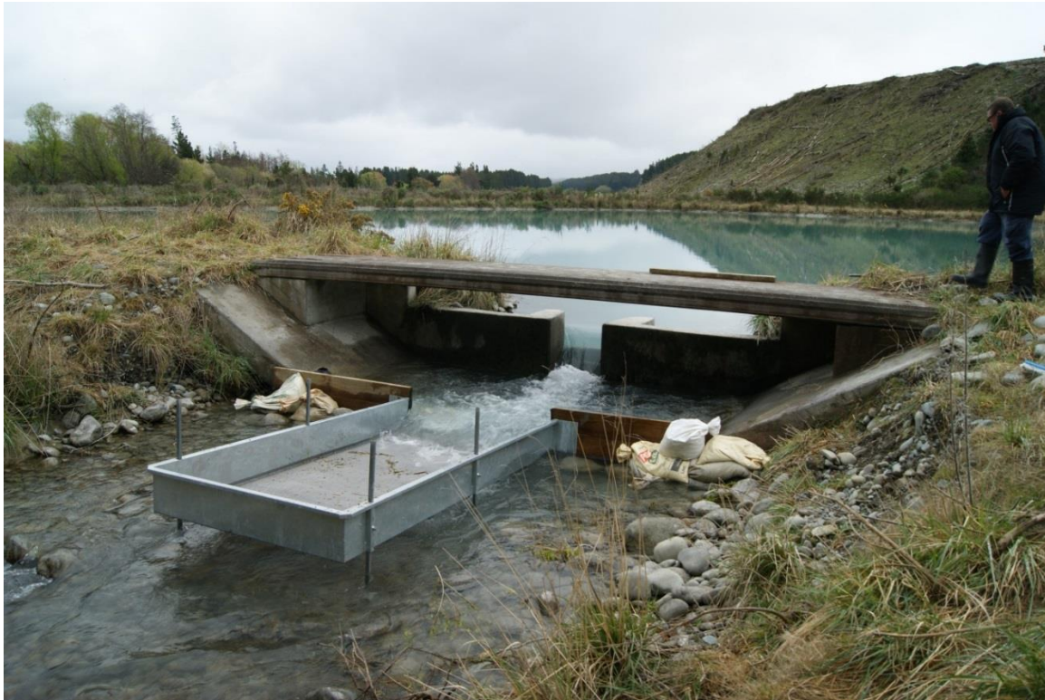
Figure 2-6: The bypass trap. This trap was installed directly in the bypass channel immediately downstream of the outlet weir.
