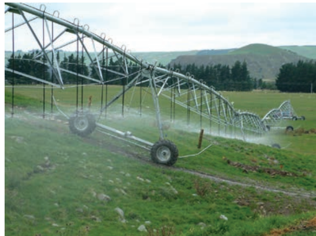
Figure 4. Very steep areas exacerbate surface run-off and apply high loads to machine components including gearboxes
