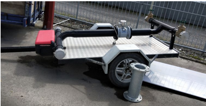
Image: An example of a simple flow rig design. The meter is in its own permanent headworks and installed to minimum of manufacturers specifications.
