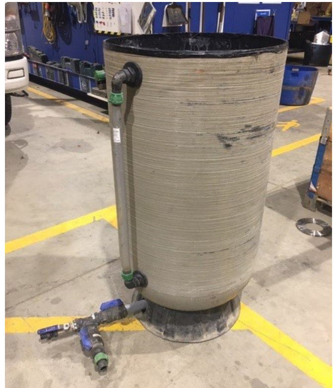
Image: A vessel which has been calibrated using scales/weight to ascertain its volume. Suitable only for very low flows and meters with low units – 1 litre or less resolution.
