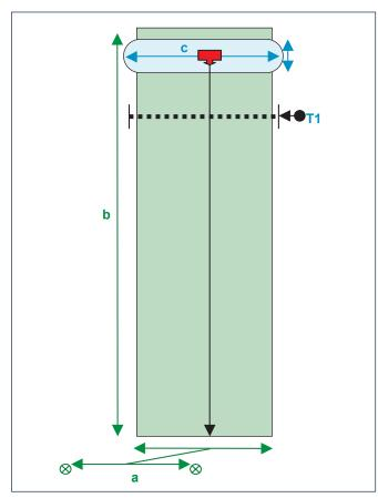
Figure 2.1. Layout of calibration test for travelling irrigators
