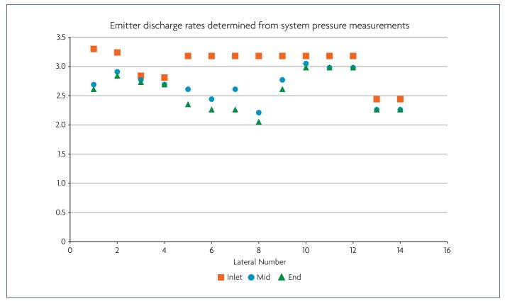
Figure 4. Emitter Discharge Rates determined from pressure measurements in driplines
