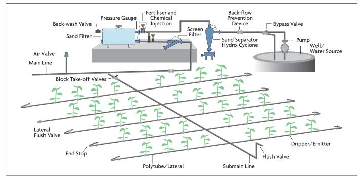
Figure C.1. Components and layout of a drip irrigation system. Based on a diagram from Jain Irrigation.
