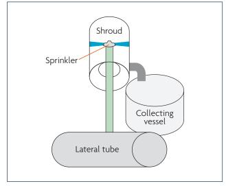
Figure 1.1. Shroud for sprayer discharge collection
