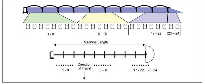
Figure 2.1. Layout of collectors along length of linear move irrigator
