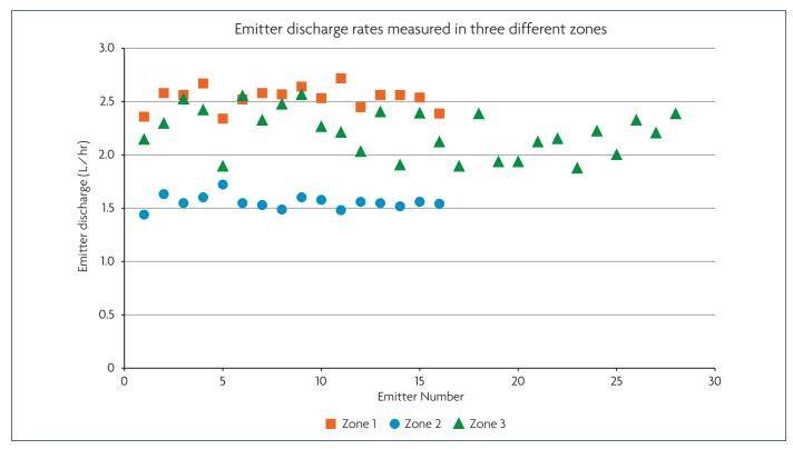
Figure 3. Emitter discharge rates measured in three different zones.
