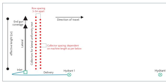
Figure 3.2. Layout of test site for linear move application testing
