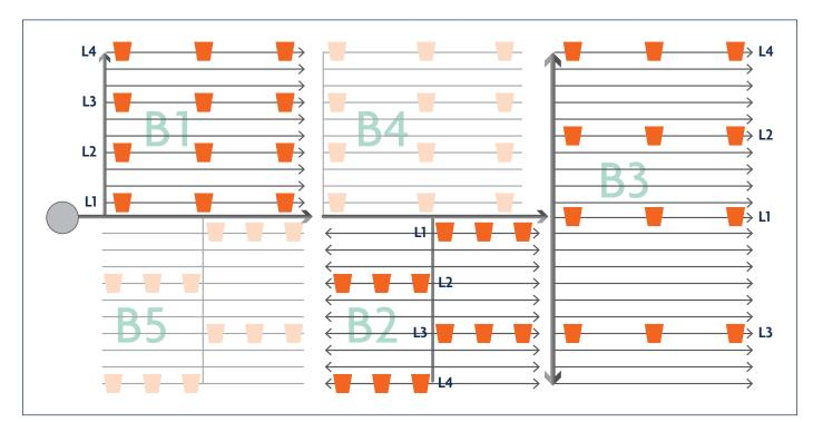
Figure 2.1. Recommended locations for emitter or sprinkler flow measurements for drip/micro irrigation calibration.
