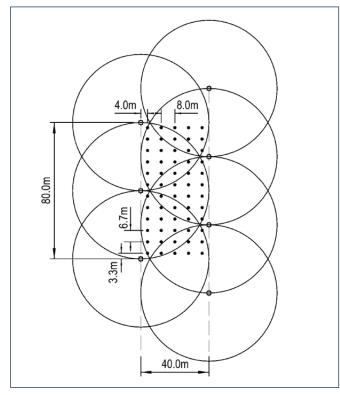
Figure 3.2. Collector spacing example.
