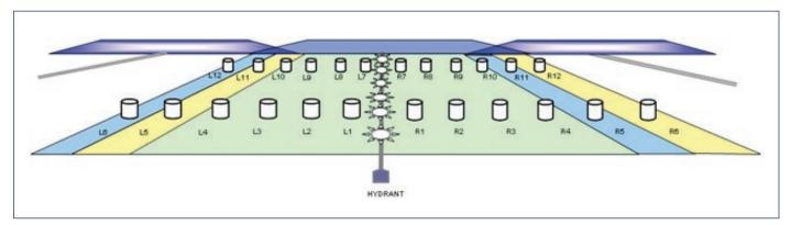
Figure 2.2. Sprayline wetted strip, overlap and collector placement
