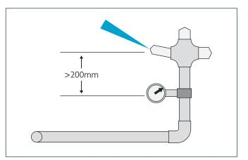
Figure 1.4. Measurement of sprinkler pressure
