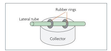
Figure 1.2. Drip-line collector
