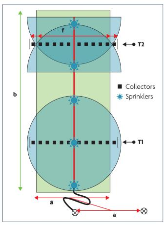
Figure 2.1. Sprayline calibration layout
