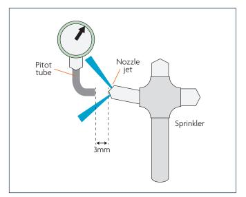
Figure 1.5. Measurement of sprinkler pressure
