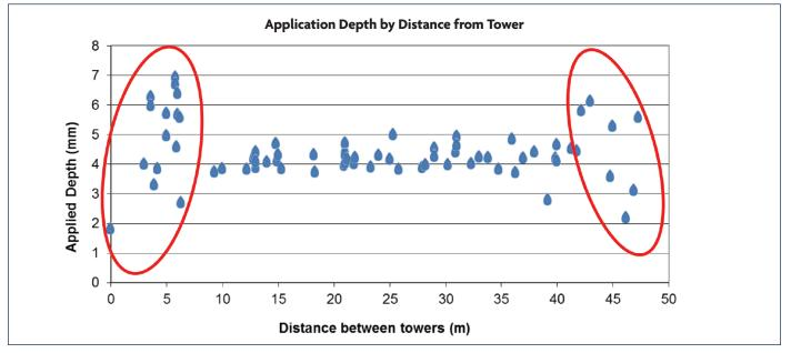
Figure 2. Application depth with all spans overlaid - catch can measurements relative to distance from towers.
