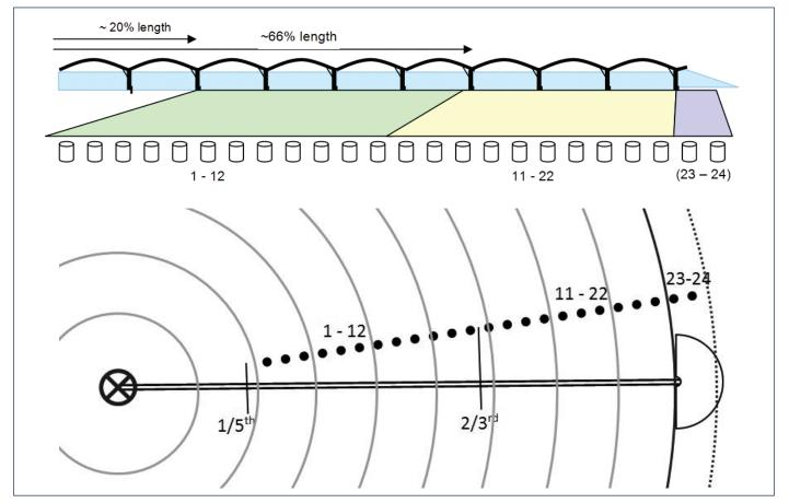
Figure 2.1. Layout of collectors along length of centre pivot irrigator.
