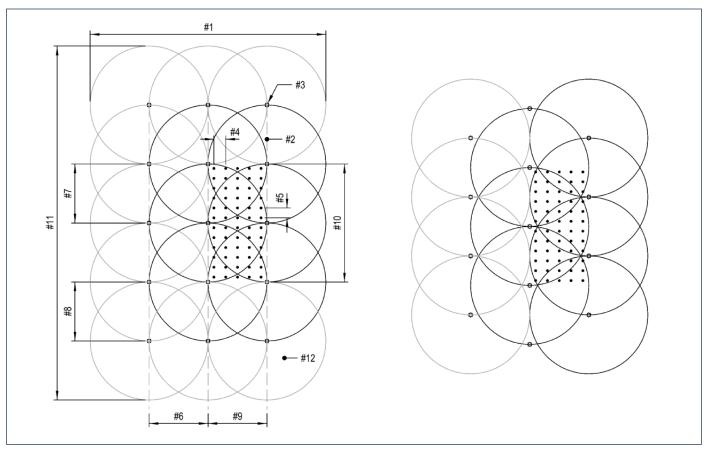
Figure 3.1. Location of sampling grid within a grid sprinkler pattern and a triangular solid-set pattern. Labels for the grid design are applicable for the triangular design
