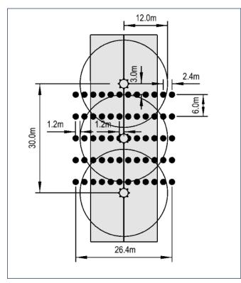
Figure 3.2. Bucket spacing example for a pod system with 15m sprinkler spacings and a 12m throw radius.
