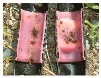
Figure 2. Dripper cut open to inspect for contaminants or other damage.
