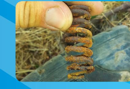
Pilot Spring corroded, affecting pressure regulation from valve.
