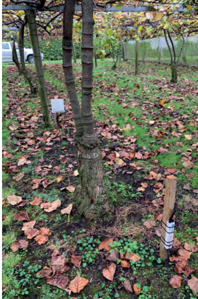
Drill and drop probe for soil monitoring.
