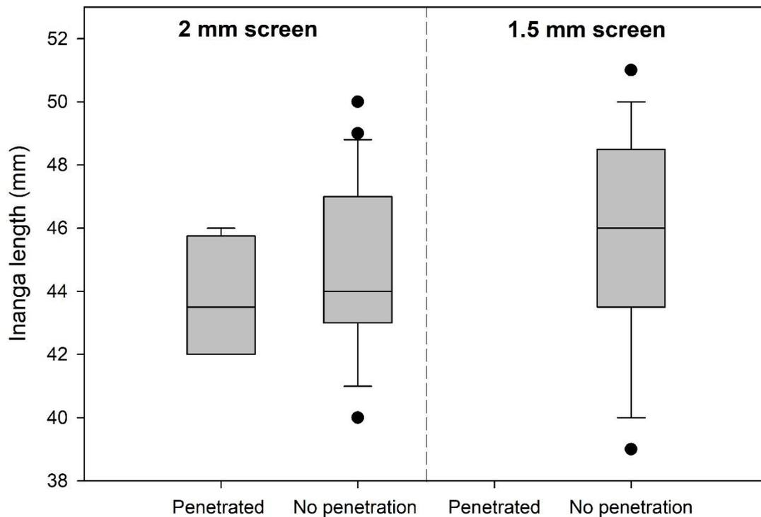
**Figure 5:** The lengths of inanga that penetrated (or did not penetrate) the 2 mm and 1.5 mm wedge-wire screens. An explanation of how to interpret boxplots is provided in the previous figure.
