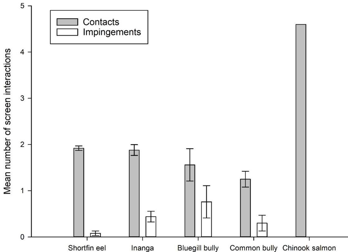
**Figure 7: Mean number ( $\pm$ SE) of screen contacts and impingements for each species tested in 2-mm wedge-wire screen experiments.** Note, separate counts were recorded if an individual fish was impinged more than once. Results for Chinook salmon should be viewed with caution as fish only interacted with the screen in one of the five replicates (which is why there is no error bar).
