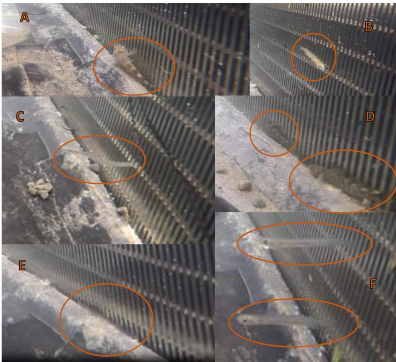
**Figure 8: Examples of screen contacts, impingements and penetrations viewed on the video footage.** Fish are circled in orange for clarity and the images show: A) common bully resting against the screen, B) īnanga impinged on the screen, C) shortfin eel attempting to penetrate the screen, D) two bluegill bullies resting against the screen, E) shortfin eel sitting next to the screen and F) two īnanga attempting to avoid the screen.
