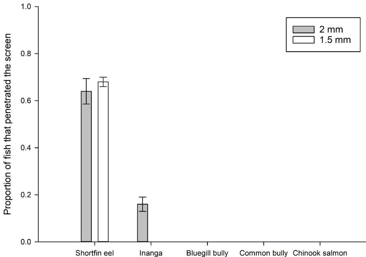
**Figure 3: Mean proportion ( $\pm$ SE) of fish species that penetrated the two different-sized wedge-wire screens.**
