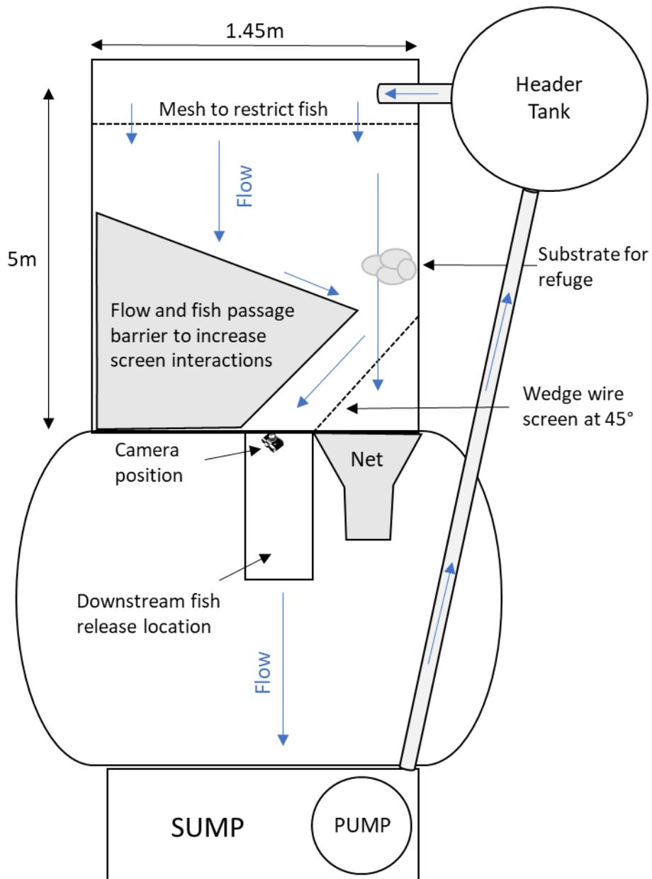
**Figure 2:** Bird's eye view schematic diagram of the outdoor stream simulator. The blue arrows indicate the direction of flow through the recirculating system.
