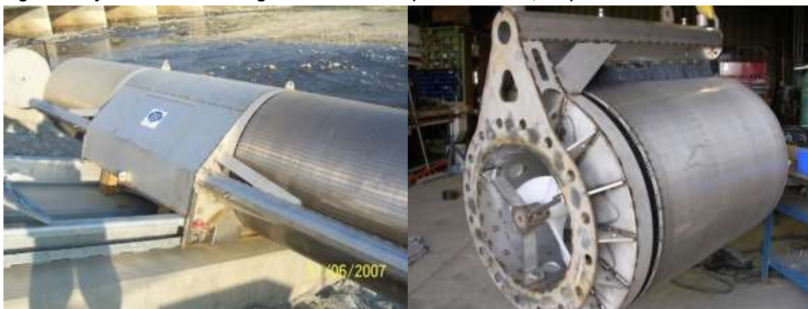
Figure 7: Cylinder Screens Design in United States (Intake Screens, Inc.)
