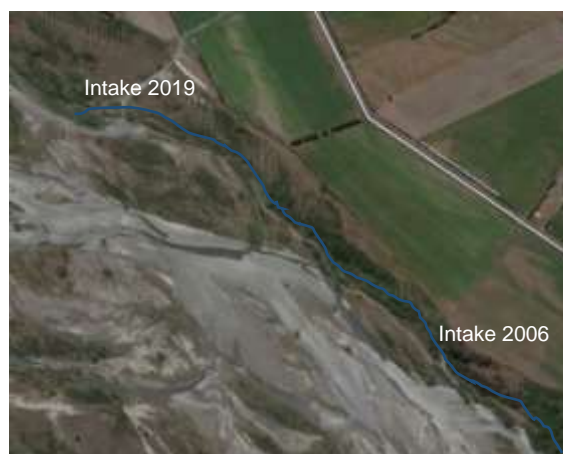
Figure 7. Same frame as Figure 6, taken in late 2019. Figures 6 and 7 indicate the degree of river morphology that alter the location of the intake.
