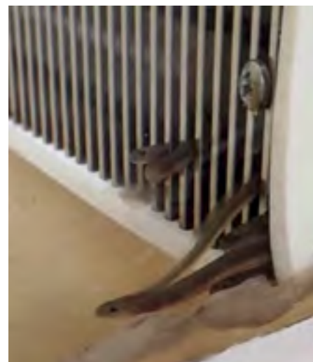
Shortfin eels would weave their bodies through the 3mm wedge-wire as a spot to rest or to utilise as cover in the flume experiments.
