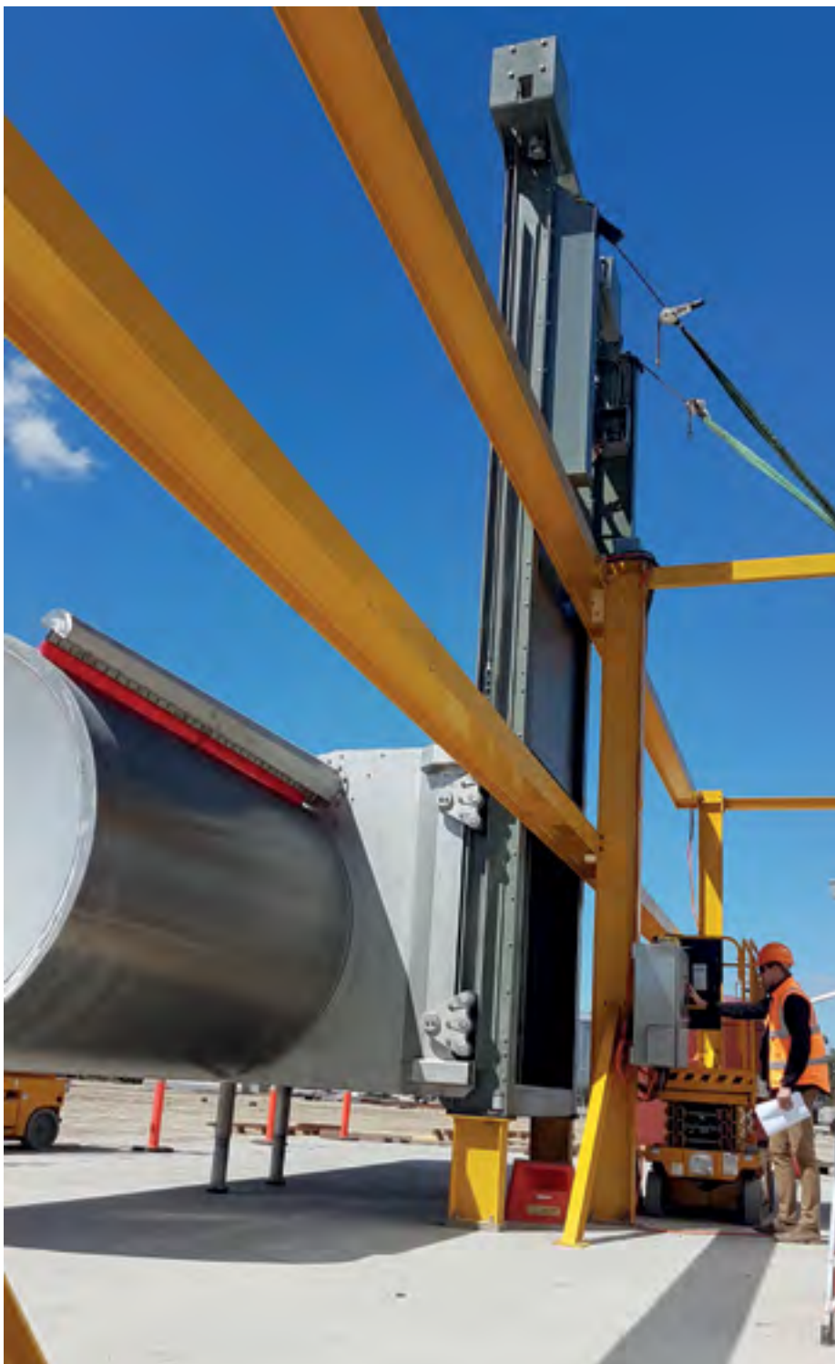
AWMA in-house factory acceptance testing of fish exclusion screen, retrieval system and isolation gate as part of the quality management system, required prior to dispatch.
