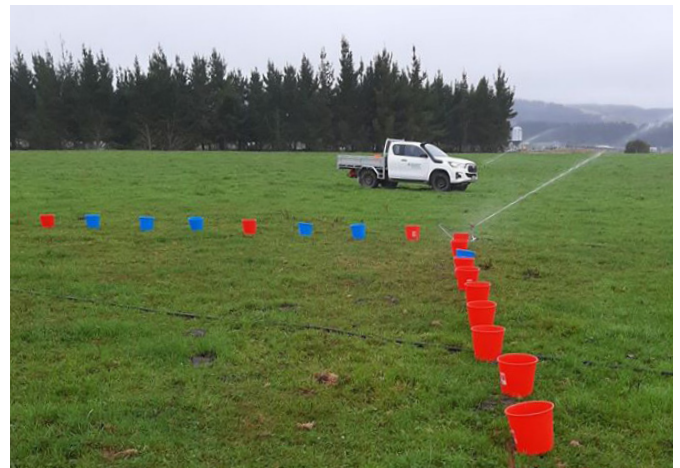
Bucket testing in Kaikōura – simple and effective
