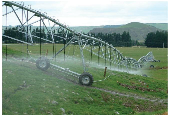
Figure 4. Very steep areas exacerbate surface run-off and apply high loads to machine components including gearboxes.
