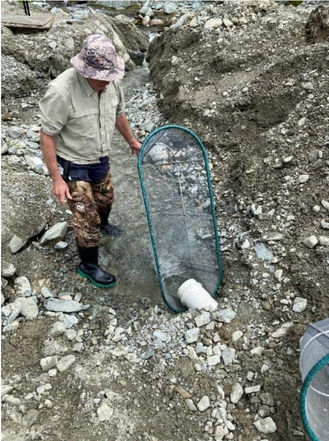
Figure 9 Rigid-framed wire mesh net on the screen bypass outlet, December 2021.
