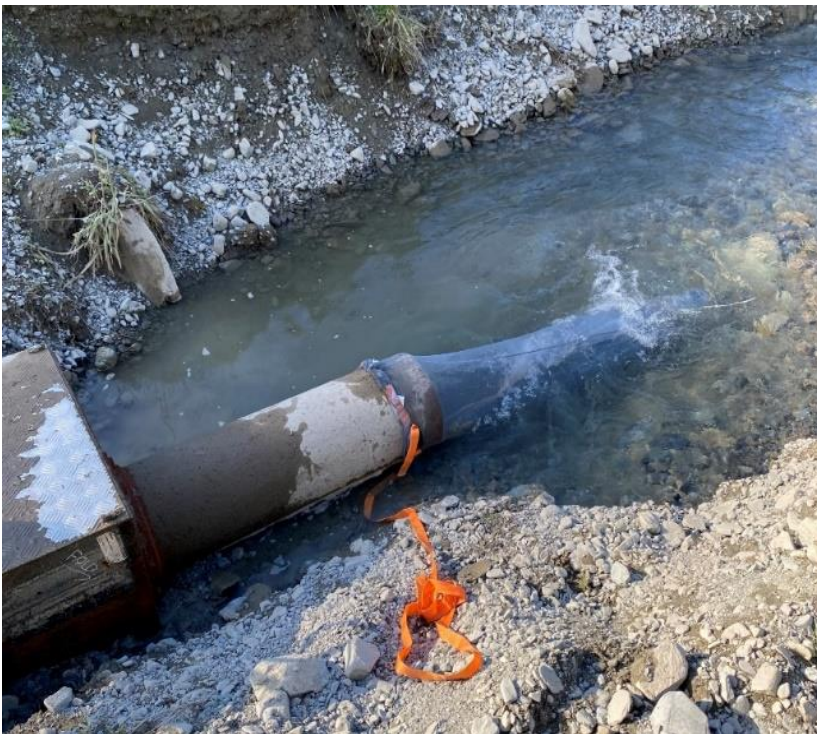
Figure 10 Custom-fitted soft mesh net with internal trap on the irrigation outlet, February and June 2022.
