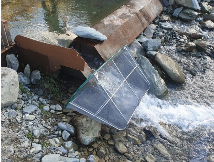
Figure 12 Rigid-framed net used on the upstream bypass outlet February and June, 2022.
