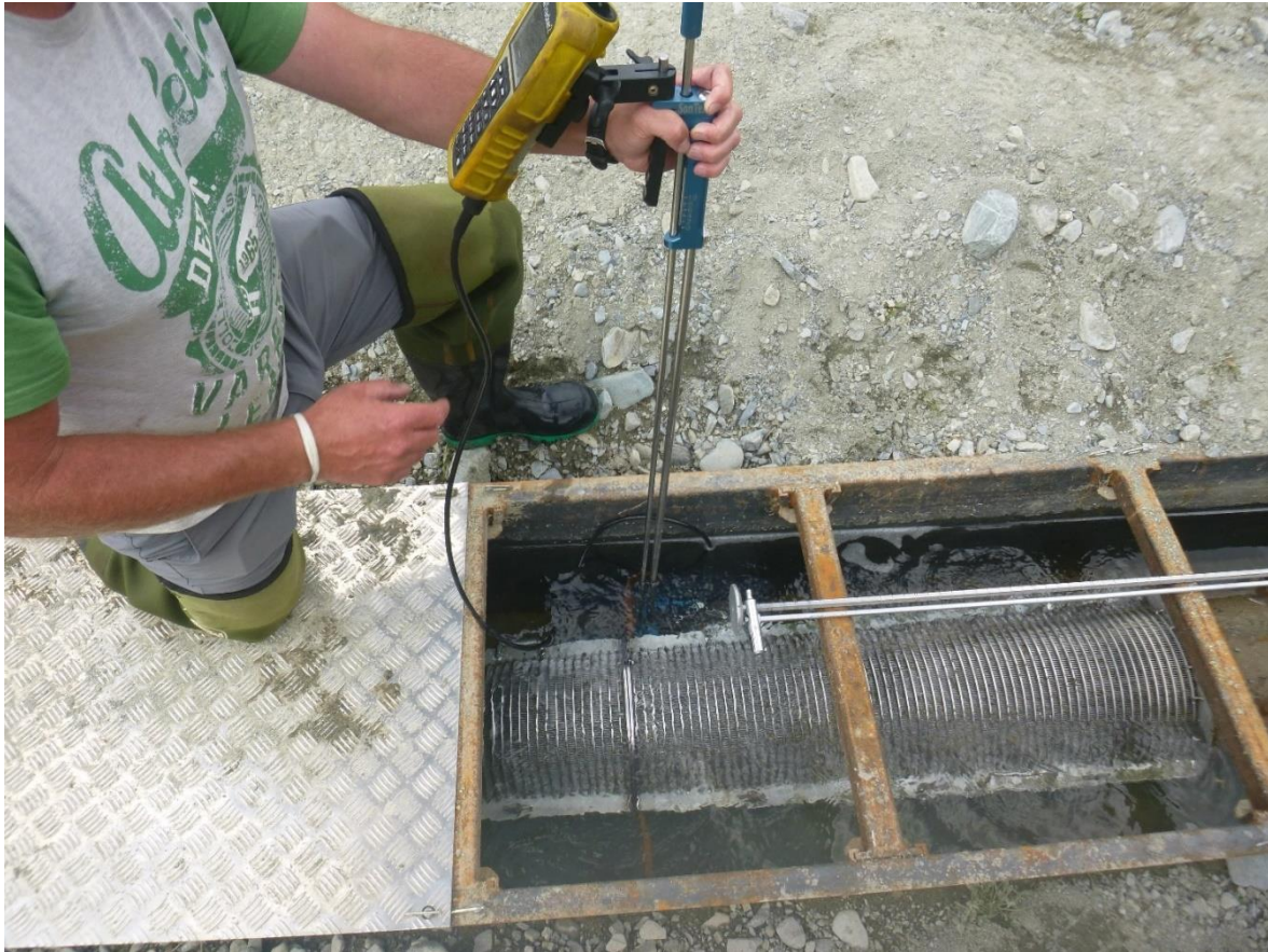
Figure 13 Measurement of irrigation intake flow 0.85m from the entrance to the screen at which point the fish screen diameter is 0.27m.
