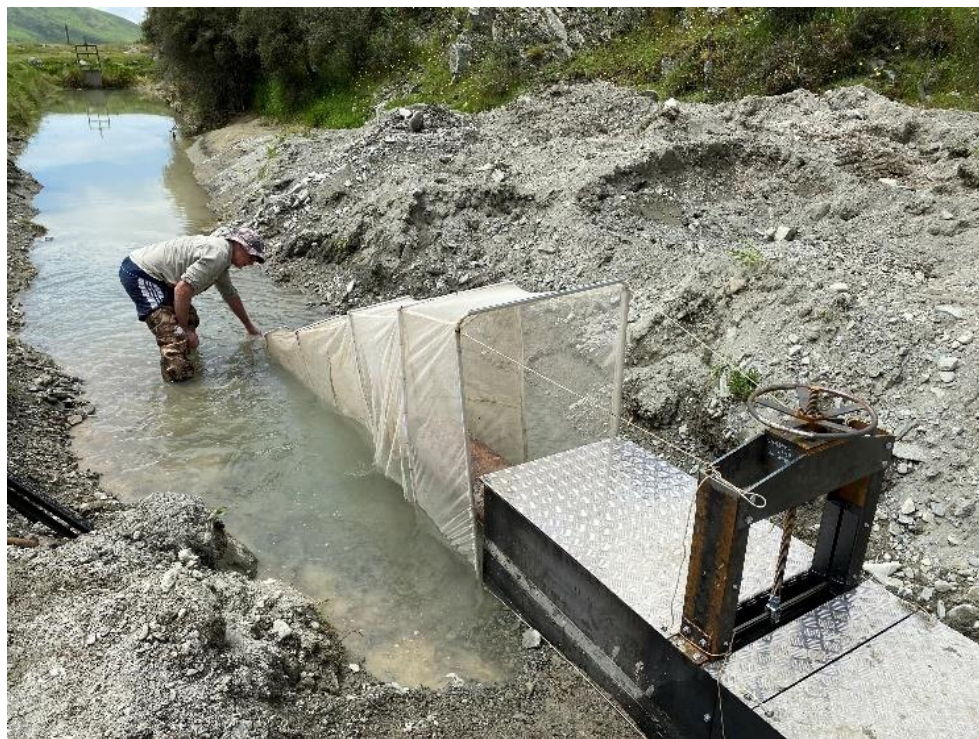
Figure 8 Rigid-framed mesh net with irrigation outlet pipe discharging into two internal non-return mesh traps, December 2021.
