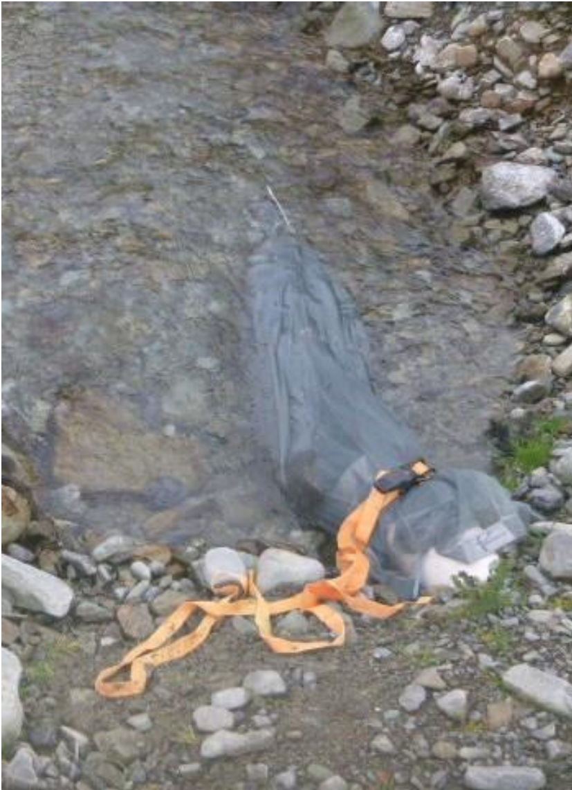
Figure 11 Custom-fitted soft mesh net with internal trap on the screen bypass outlet, February and June 2022
