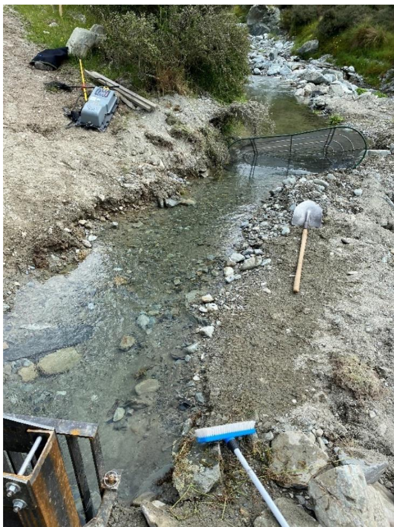
Figure 5 Intake channel upstream from fish screen and upstream "Maxi" net barrier to reduce migration of wild fish into the test area and released fish out of the test area, December 2021
