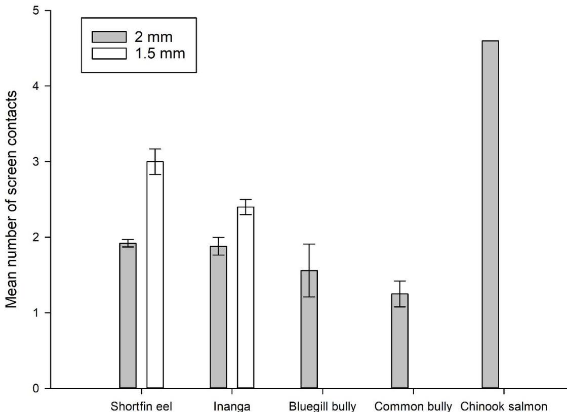
**Figure 6: Mean number ( $\pm$ SE) of screen contacts for each species for the 2 mm and 1.5 mm wedge-wire screens.** Screen contacts included fish touching the screen, resting against the screen (for less than 10 seconds) and attempting to force themselves through. Results for Chinook salmon should be viewed with caution as fish only interacted with the screen in one of the five replicates (which is why there is no error bar).
