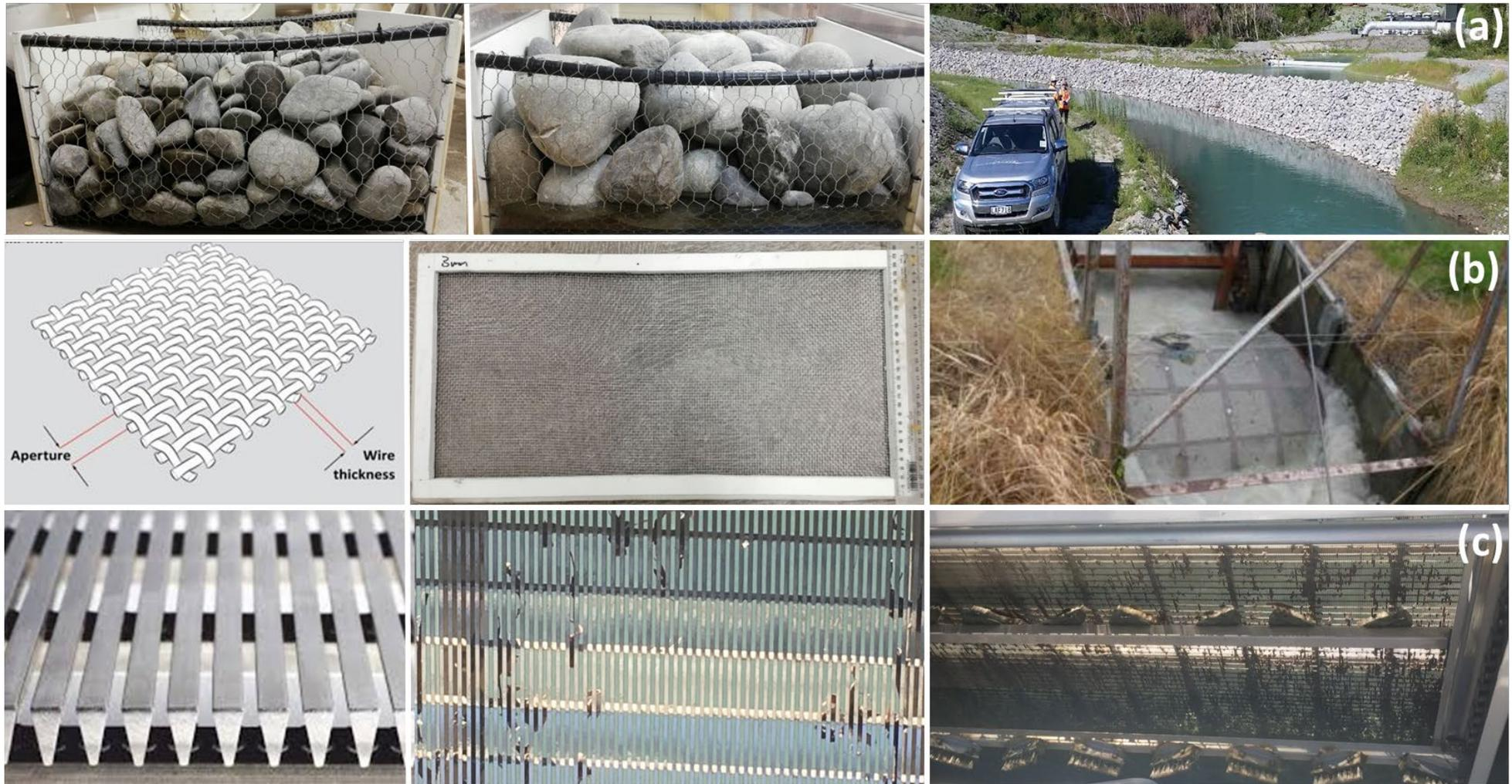
**Figure 3:** The three screen types tested in this study were: (a) rock bund, (b) woven wire mesh and (c) wedge-wire mesh. The left and centre panels show the experimental screening material used in the trials and the right panel shows examples of this material being used in New Zealand fish screens. Note, the two baskets of rocks in (a) show the 50–100 mm (left) and 100–200 mm (centre) rock treatments tested.
