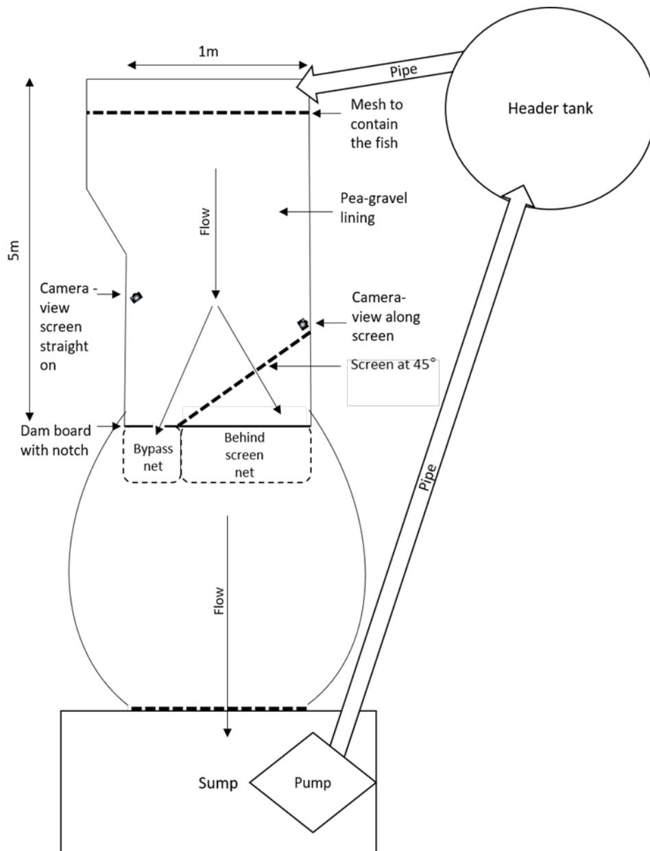
**Figure 4:** Birds eye view diagram of the outdoor stream simulator.
