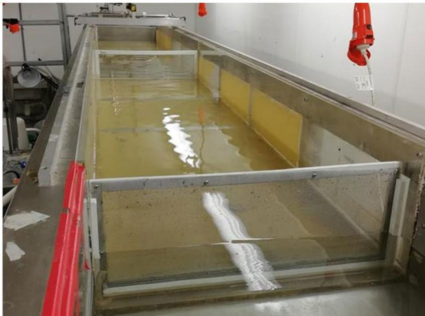
**Figure 2:** Schematic of indoor flume setup viewed from the side (top) and photograph with the downstream mesh barrier in the foreground looking longitudinally down the flume apparatus (bottom). In the bottom picture the 3 mm woven-wire mesh screen is being tested.
